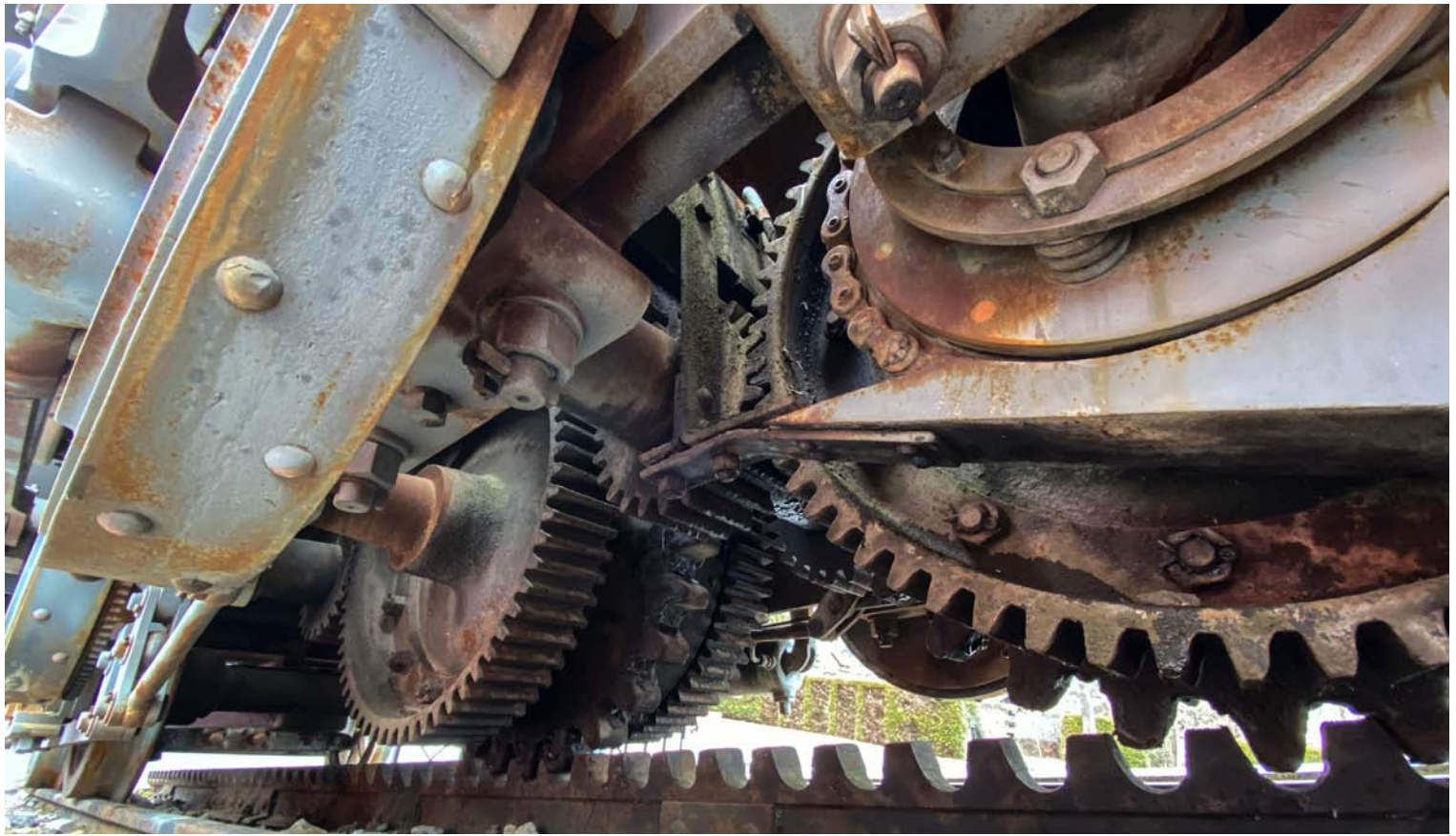
A vintage rack railway locomotive displayed in Chamonix illustrates the principle of the cog system.
